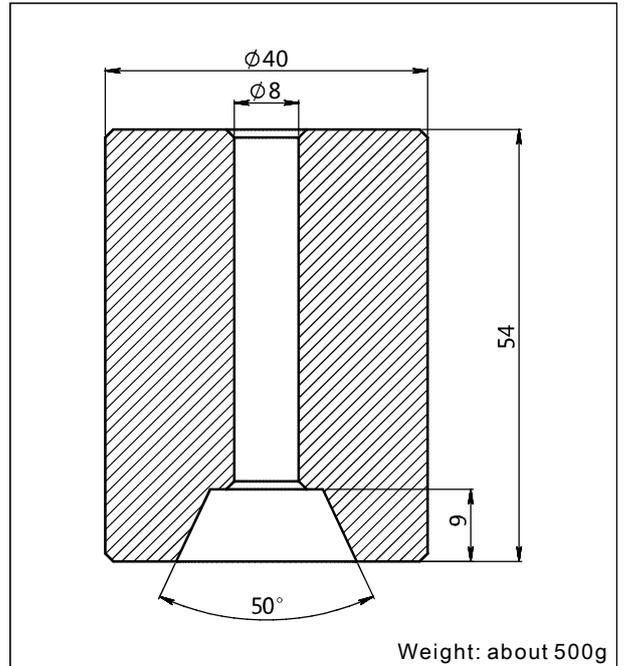
In order to prevent measurement errors caused by sideways movement of product and ensure accuracy, you can add additional counter weights by screwing together and then connecting directly to the product. Each product can be added three counter weights at the most.
