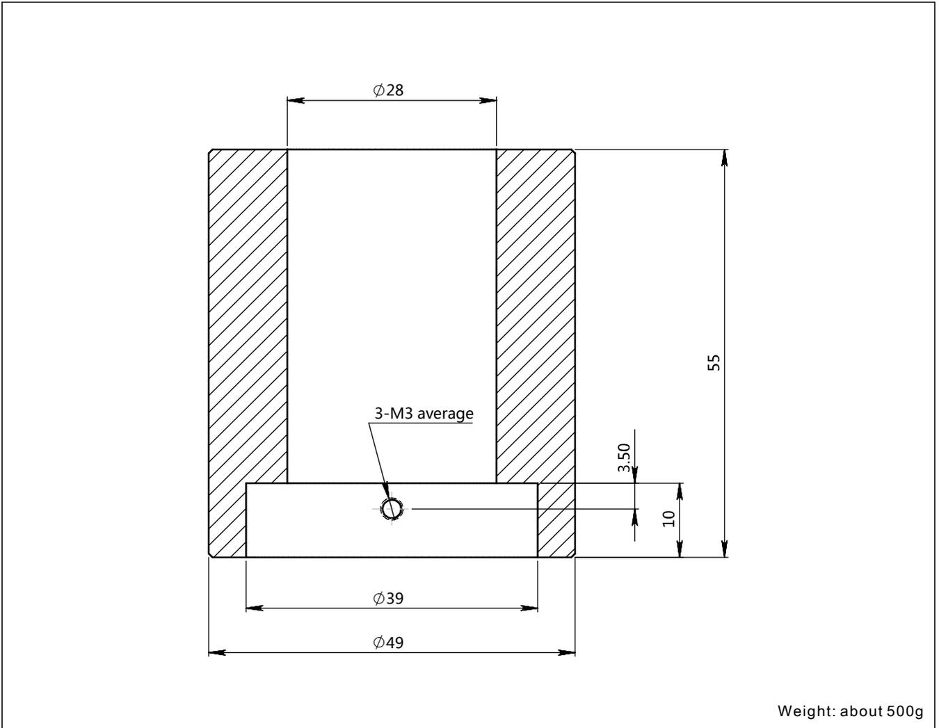
In order to prevent measurement errors caused by sideways movement of product and ensure accuracy, you can add additional counter weights by screwing together and then connecting directly to the product. Each product can be added three counter weights at the most.
