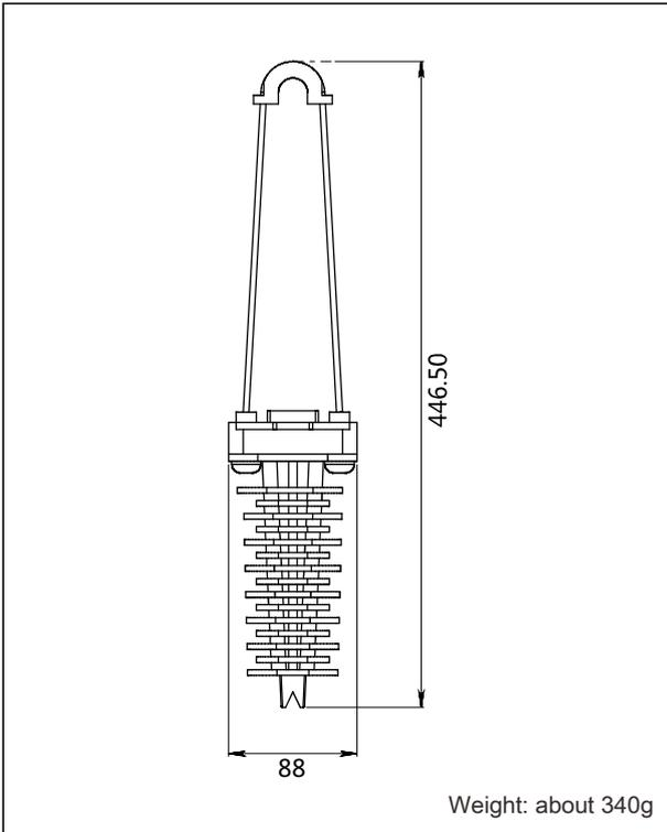
Counter weight (P5) dimension (unit: mm)
